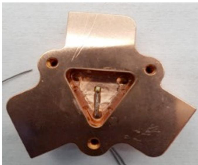
LLAMA device in LAr will monitor in time attenuation and triplet lifetime
