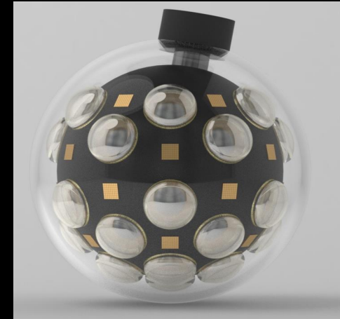
TRIDENT Hybrid DOM: 3-inch PMTs + Silicon PMs
