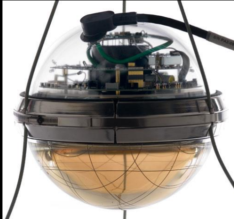
IceCube Downward-facing 10-inch PMT
