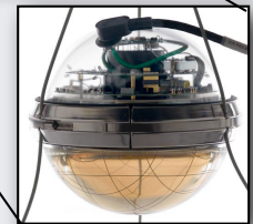
Digital Optical Module (DOM)
