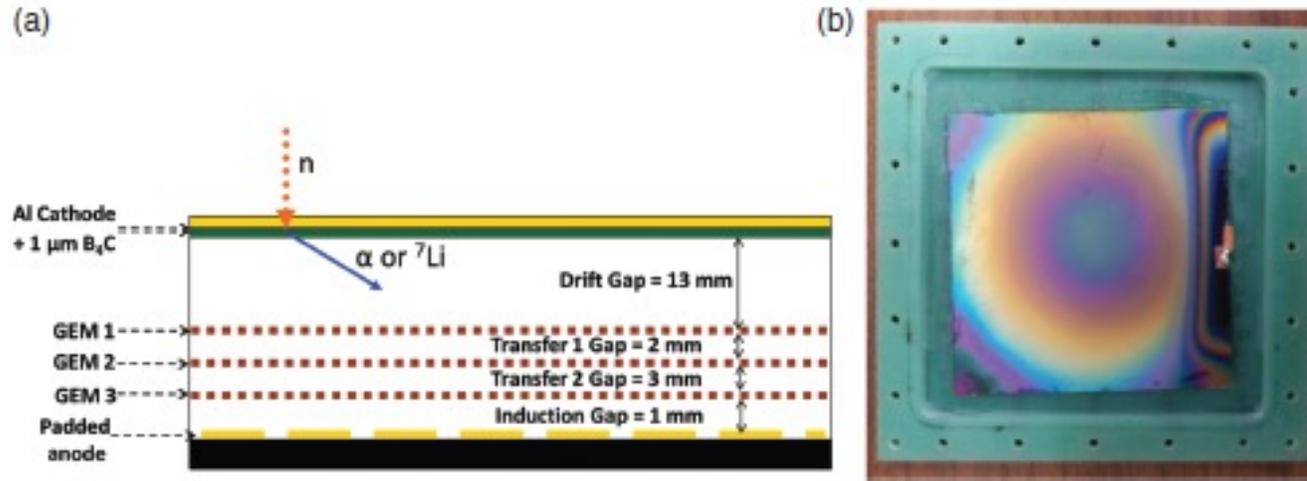
Fig. 2. (a) Detector schematics; (b) borated cathode.
