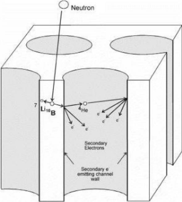
Fig. 2: Detection mechanism of the MCP-based detectors [19].
