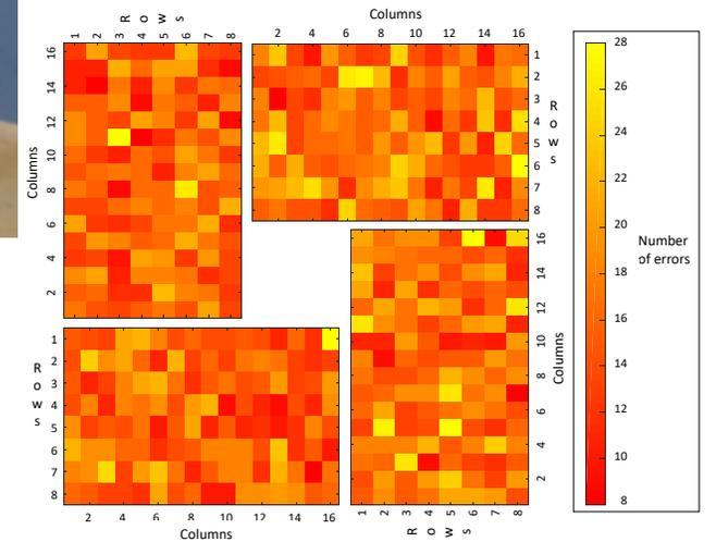
SRAM based detectors: bit flips
