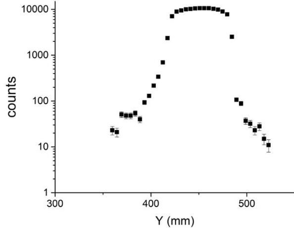
Map is measured with a diamond detector with 2 mm accuracy
