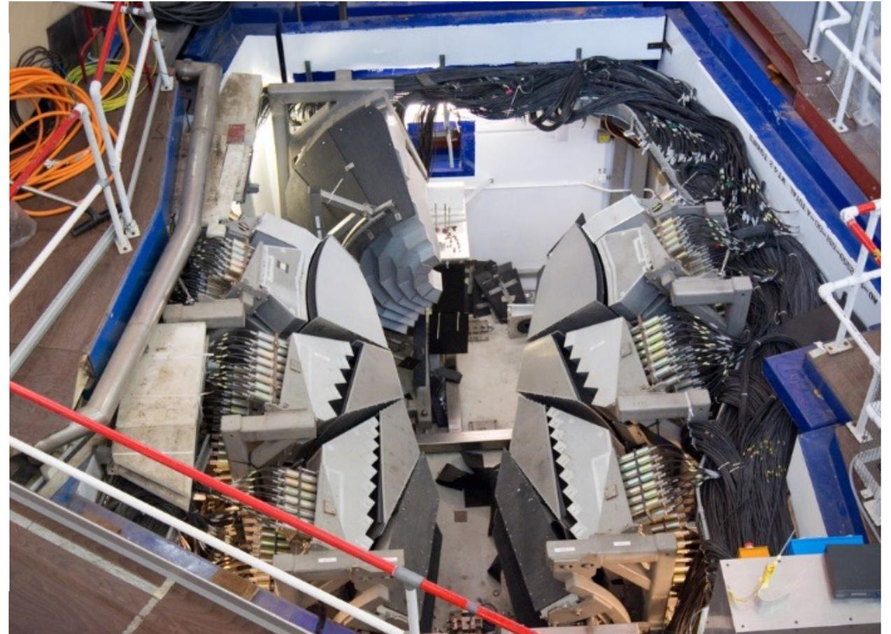
the GEM scintillator detector system contains 660,000 individual optic fibres, whose total length will be about 350 kilometres.
