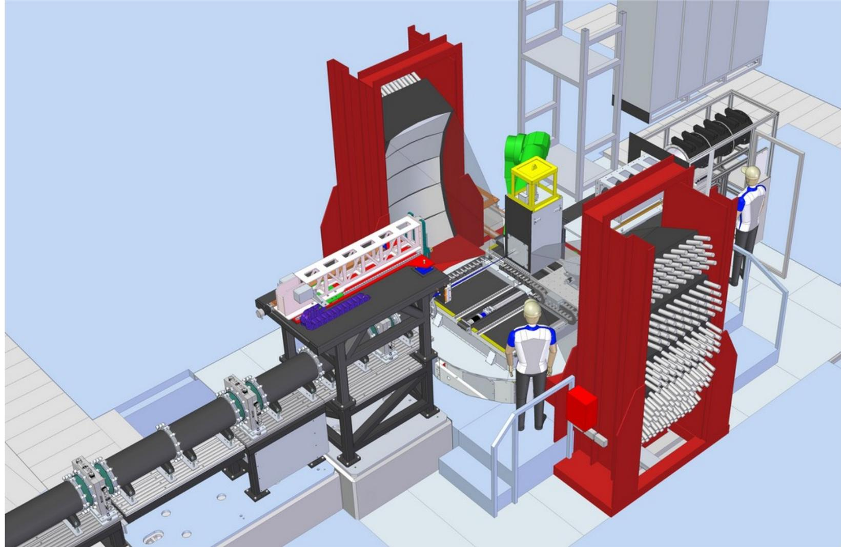
IMAT schematic with tomography camera and 90-degree diffraction detectors
