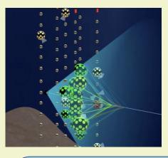
Detection mechanism Measurement of the Cherenkov light emitted by the charged product particles that result from a neutrino interaction near the detector
