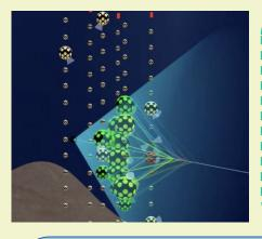
Detection mechanism Measurement of the Cherenkov light emitted by the charged product particles that result from a neutrino interaction near the detector
